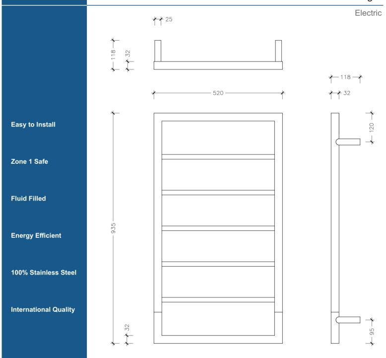
The Electrical Outlet (EO) is through either the bottom left or right hand bracket, 95mm up from the bottom of the rail. The EO is to be specified at time of confirming the order.
