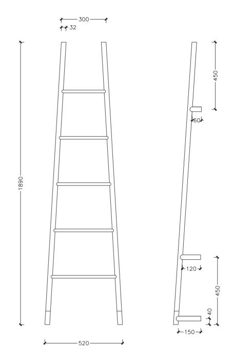
The Electrical Outlet (EO) is through either the bottom left or right hand bracket, 40mm up from the bottom of the rail. The EO is to be specified at time of confirming the order.
