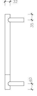
The Electrical Outlet (EO) is through either the bottom left or right hand bracket, 40mm up from the bottom of the rail. The EO is to be specified at time of confirming the order.
