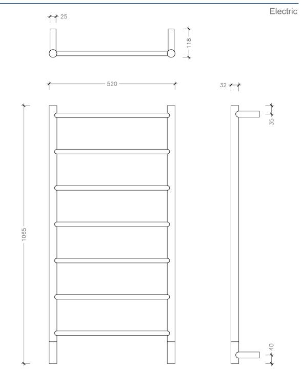
The Electrical Outlet (EO) is through either the bottom left or right hand bracket, 40mm up from the bottom of the rail. The EO is to be specified at time of confirming the order.
