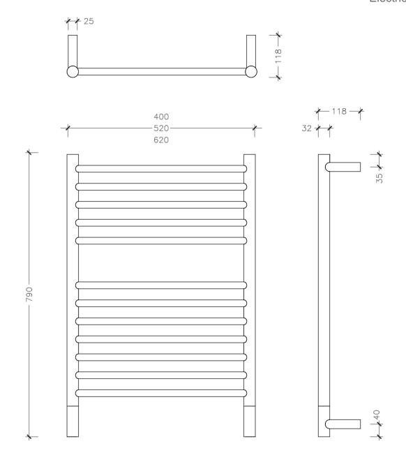
The Electrical Outlet (EO) is through either the bottom left or right hand bracket, 40mm up from the bottom of the rail. The EO is to be specified at time of confirming the order.
