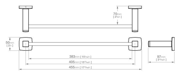
Dimensions given are in mm and inches. LIQUIDRed® reserves the right to alter and /or remove designs from time to time without prior notice.
