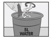
Mix 20kg **TAL GOLDSTAR 6** with 5L of cool, clean water. Using a mechanical mixer, mix to a creamy lump-free paste, while adding powder.
