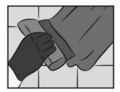
Grout after 4 hours with **TAL Grout** (as per instructions on the grout bag). Full service after 6 hours when using **TAL Goldflex Grout**.
