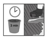
Let stand for 3 minutes, then stir again. Use within 90 minutes (pot life). Apply adhesive with a suitable notched trowel. Ensure the tile is in full contact with the adhesive. Apply only as much as can be tiled in 10-15 minutes.
